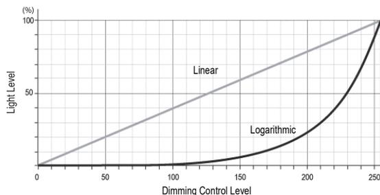
Dimming parameters can be changed using Tridonic masterCONFIGURATOR software.
