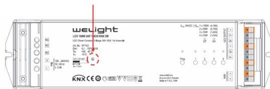
Compliance with the maximum permissible reference temperature at the tc point must be checked under operating conditions in a thermally stable state. The maximum value must be determined under worst-case conditions for the relevant application.
