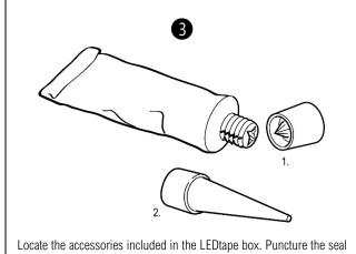
of the tube using the backside of the tube cap. Screw the dispersion needle onto the tube. Cut the top of the needle at an angle of 45-60°.
