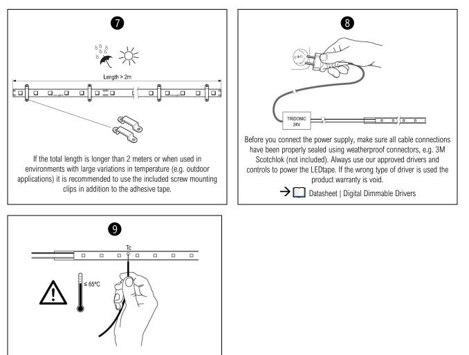
The temperature on the surface of the LEDtape (tc) may under no circumstances be higher than 65 °C if the expected lifetime of the LEDtape is to be met.
