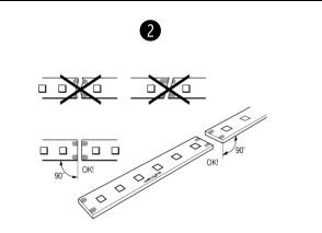
Always cut the LEDtape in a straight line - 90° in relation to the PCB edges. Failure to do so can result in damage of the internal conducting paths. Use Welight's official connection accessories to split, connect, bridge and re-seal the LEDtape.
