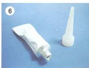
6-7. Put the needle on the top of glue tube, cut the top of the needle at an angle of 45-60 degrees.
