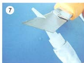
6-7. Put the needle on the top of glue tube, cut the top of the needle at an angle of 45-60 degrees.
