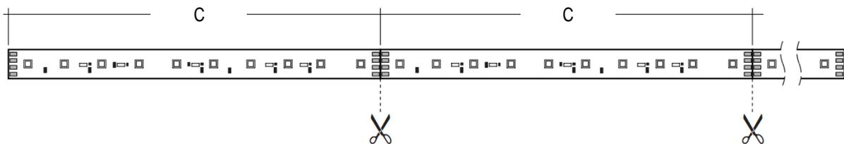
It is recommended to use the connection accessories listed in section *Accessories* to split, connect and bridge the LED-tape.
