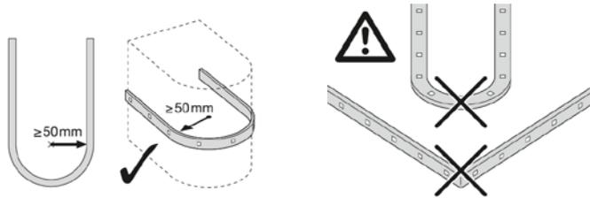
The LED module itself and all its components must not be mechanically stressed. When fixing the LED-tape to a surface, apply an even but gentle pressure and try to avoid applying pressure directly on the LED itself (the maximum allowed pressure is 20 N/cm<sup>2</sup>).
