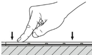
After assembly always check that the entire length of the tape has attached properly to the surface and that there is no air pockets underneath the PCB.
