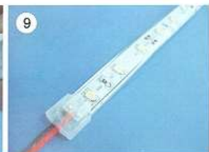
8-9. Dispense the glue on the gap between the end-cap and LED strip, and the small hole on the end-cap. Please wait for 30 minutes till the glue gets solidified.
