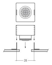
With long mounting clamps the sensor can be adjusted up or down so the sensor edge is flush with the surface of the luminaire.
