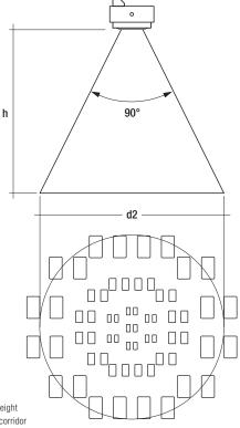
The recommended maximum room height for office applications is 3 m and for corridor applications for example 4 m.
