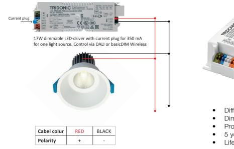
Dimmable constant current LED driver with simple digital control via DALI plus a rotary dimmer or via Bluetooth with basicDIM Wireless. Compact design for narrow installations with optional strain-relief for remote installation.
