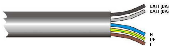
Figure: Typical texture of used wires
