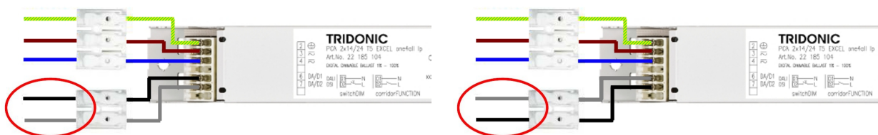
Figure: Different polarity of DALI lines
