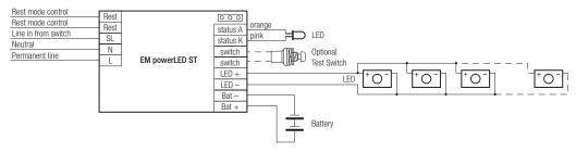
Take care that the LED is connected with the right polarity. LED that are connected to the EM powerLED devices should have a reverse polarity protection device such as a schottky diodes fitted, otherwise irreversible damage could occur if the LED is connected in reverse polarity. Any protection device must be capaple of handling in excess of 700 mA.
