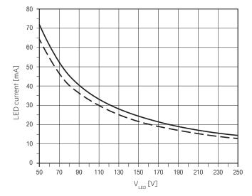
EM converterLED BASIC 205 NiCd/NiMH 250V Article number: 89800564 6.0 V battery voltage
