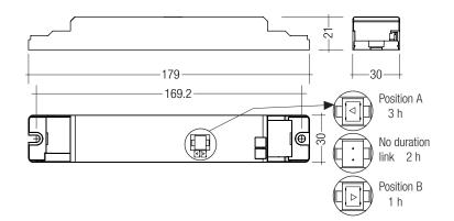
Note: LED Driver supplied with duration link in 3 hours position. Duration link must be set before battery and mains connection.
