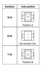
Module supplied with duration link in 3 hours position (position A).
