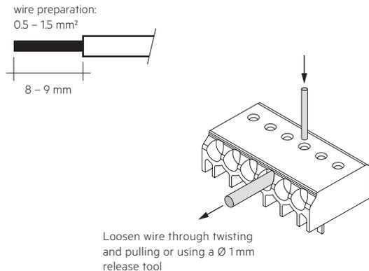
**Wiring type and cross section**
