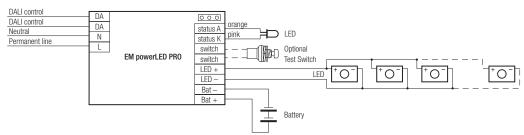
Take care that the LED is connected with the right polarity. LED that are connected to the EM powerLED PRO EZ-3 devices should have a reverse polarity protection device such as a schottky diodes fitted, otherwise irreversible damage could occur if the LED is connected in reverse polarity. Any protection device must be capaple of handling in excess of
