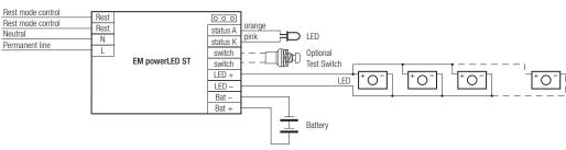
Take care that the LED is connected with the right polarity. LED that are connected to the EM powerLED PRO EZ-3 devices should have a reverse polarity protection device such as a schottky diodes fitted, otherwise irreversible damage could occur if the LED is connected in reverse polarity. Any protection device must be capaple of handling in excess of 1,000 mA.
