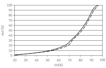
Remark: Dimming curve based on DIMMER ELKO 315GLE!
