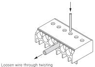
Loosen wire through twisting and pulling or using a Ø 1mm
