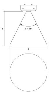
The recommended maximum room height for office applications is 3 m and for corridor applications for example 4 m. Up to 2 m mounting height presence is detected and over 2 m motion is detected.
