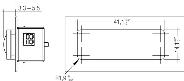
**Mounting in luminaire housing with Mounting Kit:**
