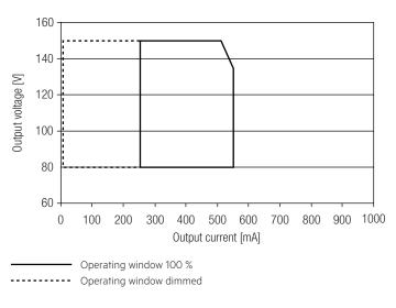
Make sure that the LED Driver is operated within the given window under all operating conditions. Special attention needs to be paid at dimming and DC emergency operation as the forward voltage of the connected LED modules varies with the dimming level, due to the implemented amplitude dimming technology. Coming below the specified minimum output voltage of the LED Driver may cause the device to shut-down. See chapter "6.11 Light level in DC operation" for more information.
