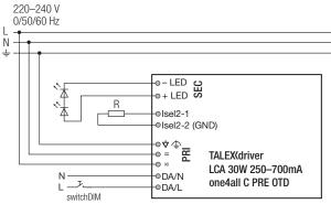
For wiring in dimming operation with ready2mains refer to the ready2mains Gateway data sheet.
