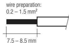
**Wiring type and cross section basicDIM Sensor 5DPI 14f**
