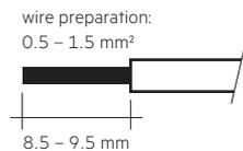
**Wiring type and cross section basicDIM Sensor 5DPI 14rc**
