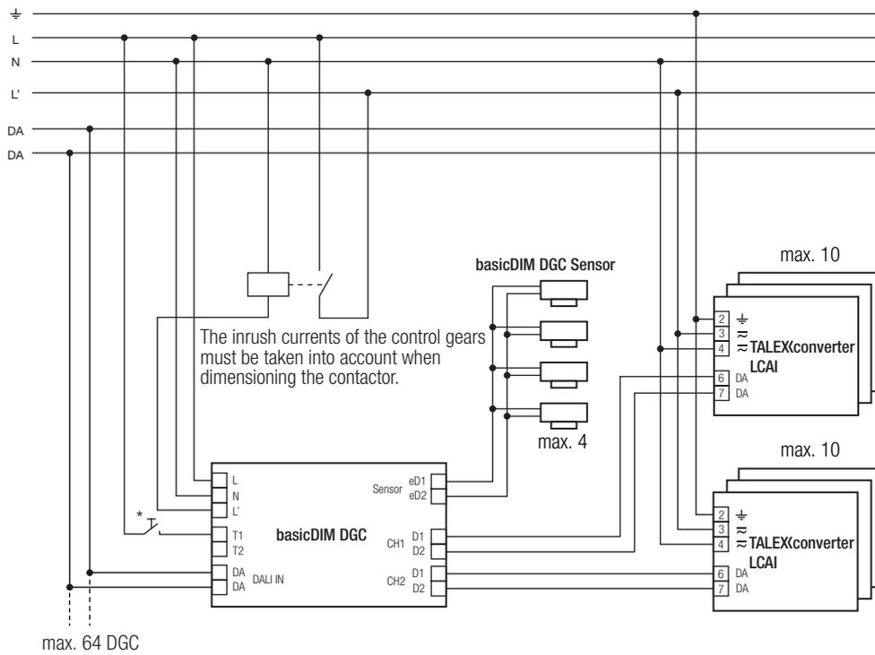
Wiring diagram basicDIM DGC with DALI PS1(2)
