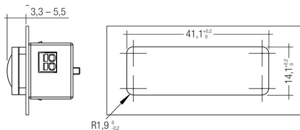
**Mounting in luminaire housing with Mounting Kit:**
