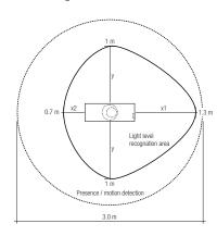
The recommended maximum room height for office applications is 3 m and for corridor applications for example 4 m. Up to 2 m mounting height presence is detected and over 2 m motion is detected.
