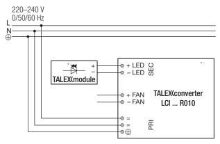
Secondary switching of LEDs is not allowed and may cause damage to the LEDs. The hot plug-in of LEDs during normal operation may result in current peaks of up to 50 % above the typical output current.
