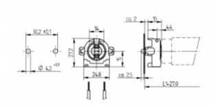
L1+27.0: Recommended dimension is based on use of one lampholder with and one lampholder without spring. The final distance should be governed by the dimensions of the respective lamps and luminaires.
