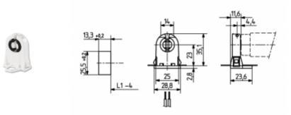
L1-4: Recommended cutout spacing . "L1" distance is determined by the length of the respective lamp.
