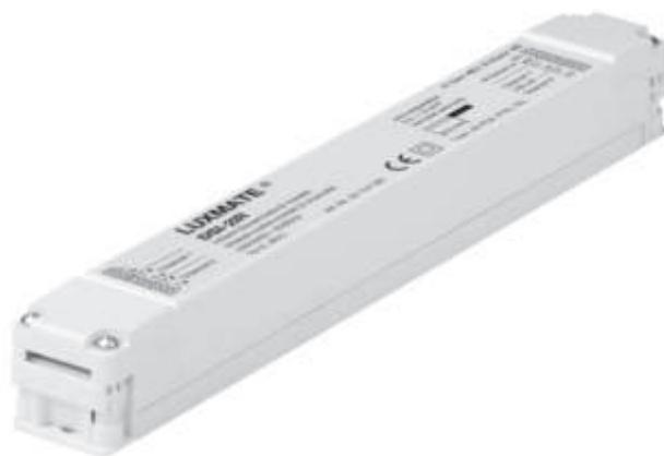
The infra-red control module DSI-2IR allows the control of 2 luminaire groups with each up to 25 digital electronic ballasts PCA, phase cutting dimmers PCD and electronic transformers TE one4all via the infra-red remote control IRS.
